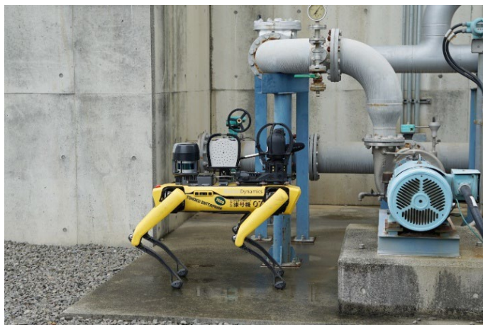
Four-legged walking robot collecting asset data during PoC testing at the Sakai Refinery
