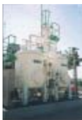
Hydrocarbon vapor recovery unit
