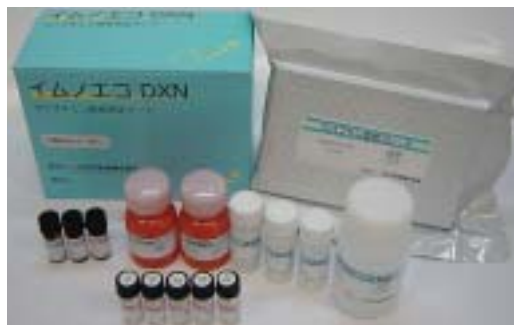
Basic dioxin test kit "Imuno-Eco DXN"
