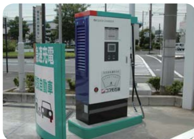
High-speed recharger for electric vehicles
