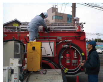
Refueling using a portable emergency pump 2
