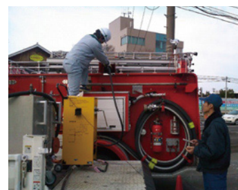
Refueling using a portable emergency pump 2
