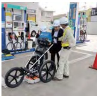
▲ Survey using ground radar
