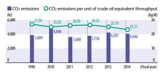
Note: In addition to the figures shown in the graph, N2O released from the catalyst regeneration tower amounted to 18 kt of CO<sub>2</sub> equivalent in fiscal 2014
