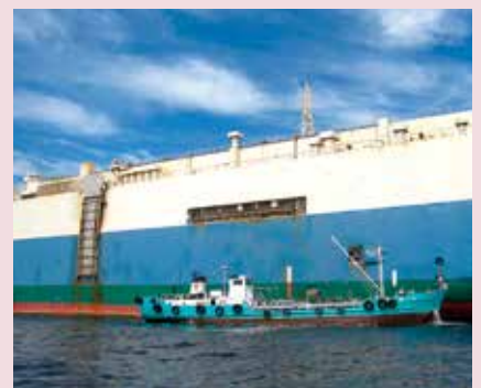
Refueling a large marine vessel at sea (fueling vessel in the foreground).
