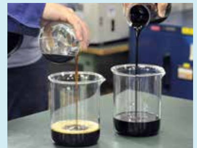
In October 2014, Cosmo Oil became the first Japanese company to import condensate from U.S. shale wells to Japan, moving to further diversify its oil products. Condensate (shown at left) is a type of crude oil yielded from gas wells as a liquid, which foams because of its high gravity and low viscosity.
