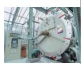
Experimental plant for slurry method biotechnological soil remediation
